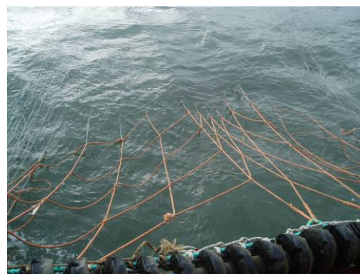
Figure 2. The large rope meshes (2.4m) at the front parts of the Eliminator trawl
